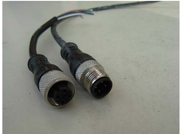
internal view after the dust test – no dust presence
