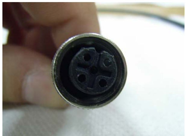
internal view of female connector after separation from the male connector
