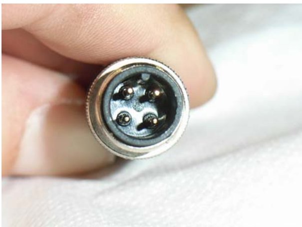
internal view of male connector after separation from the female connector
