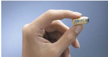
Pill-Cam™, the camera in a pill for diagnosing intestinal disease, invented by Israel's Given Imaging
