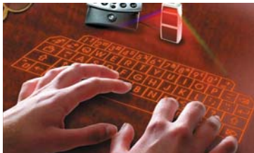
Infrared Virtual Keyboard invented by Israeli company VKB
