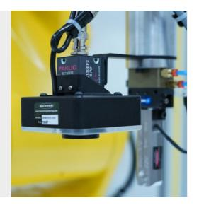
**Fenceless Collaborative Robot -** The FANUC CR-7*i*A collaborative robot includes a very sensitive built-in sensor allowing it to work safely alongside people.
