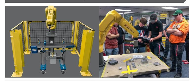
**Robot Pedestal -** Heavy duty, welded structural steel, powder coated pedestals for LR Mate robots. Available in five different heights of 24", 30", 36", 42", and 48".
