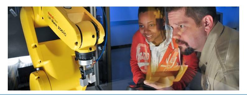
**Fenceless LR Mate -** The FANUC LR Mate 200*i*D/4S fenceless education cart combines FANUC's DCS position and speed check software with a mini safety laser scanner. FANUC's fenceless cart fits through a standard door and runs off 110V power. The fenceless cart provides a larger work envelope and introduces students to FANUC's and Allen-Bradley's integrated safety products.
