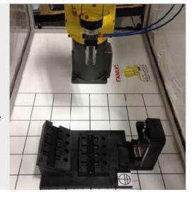
**Spot Weld -** The spot education cart simulator offers training to operate FANUC robots equipped with SpotTool software and a simulated pedestal-mount servo spot weld gun.
