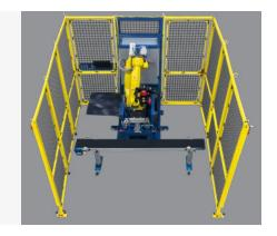
**Connected Smart Manufacturing -** Demonstrates a variety of functions on a system's HMI that require security clearance including: VFD frequency setup; recipe management system; inspection limits; I/O link setup; login; and system security settings.
