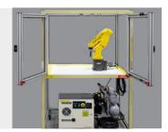
**K-12 Introductory Robotics Package -** A material handling teach pendant that connects to your computer with ROBOGUIDE software. Install, move and program a virtual robot.
