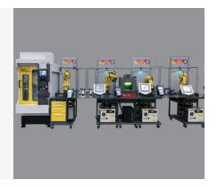
Machine Tending Educational Cell - ROBODRILL with 2D iRVision - Students familiar with CNCs or robots can learn advanced automation integration on this fenceless cell that includes an area scanner for front or side loading.
