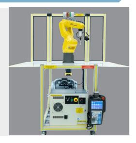
**2D** *i*RVision - *i*RVision finds parts and their precise position and orientation (X,Y, Z and R). As a result, production flexibility increases because expensive positioning fixtures are not required. 2D vision is suited for any material handling application including palletizing and depalletizing, as well as vision inspection.
